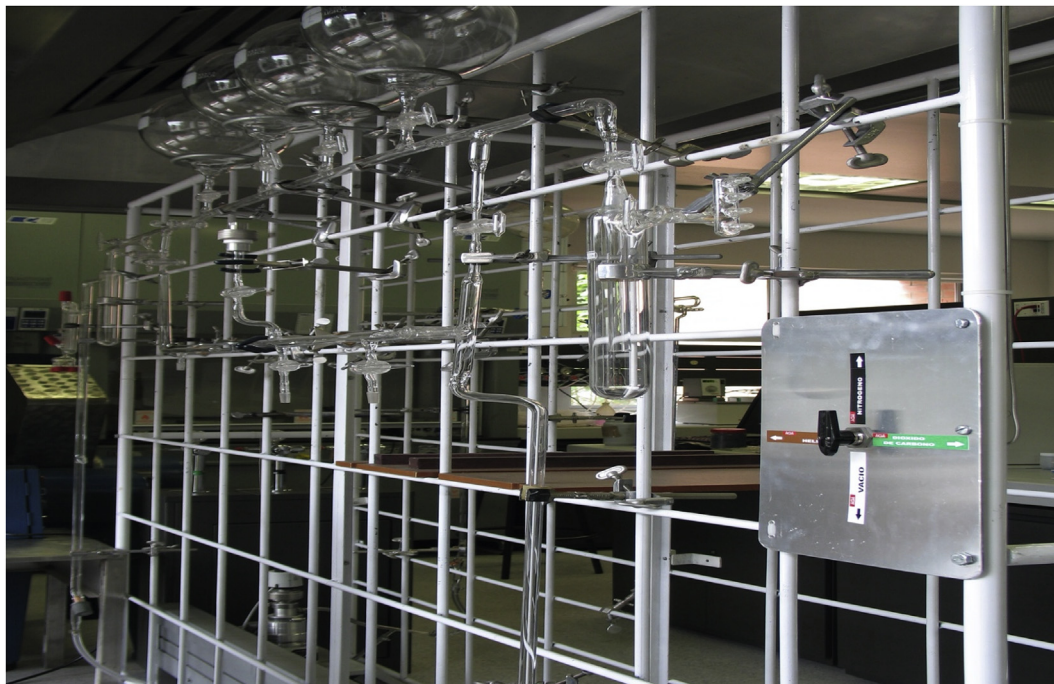
Volumetric adsorption equipment that was designed, assembled and calibrated with Paco's help in 2006.
